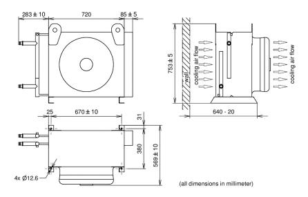
**NOTICE** Ensure unobstructed air circulation to avoid overheating. Free space on the suction side is required.
