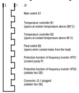
The internal interlock loop complies with the requirements for Electrical energy Source class 1 (ES1 type according to IEC 62368-1, safe separation, proof voltage resistance 4 kV ACpk to primary circuit).
