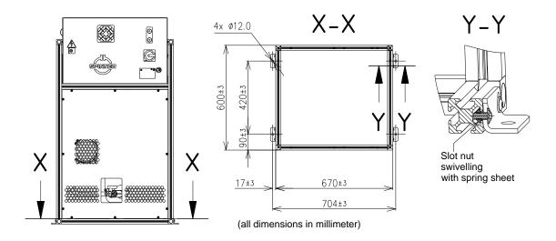
Use all 4 mounting holes of the external heat exchanger to fix it with suitable screws to the floor, or with fasteners, (e.g. wall hanger supports lengths 640 mm, refer to chapter "Accessories") and screws to a wall or support structure with bearing capacity higher than 70 kg.
