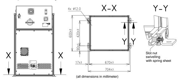
• Use all 4 mounting holes of the external heat exchanger to fix it with suitable screws to the floor, or with fasteners, (e.g. wall hanger supports lengths 640 mm, refer to chapter "Accessories") and screws to a wall or support structure with bearing capacity higher than 70 kg.
