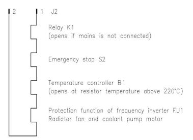
The internal interlock loop complies with the requirements for Electrical energy Source class 1 (ES1 type according to IEC 62368-1, safe separation, proof voltage resistance 4 kV ACpk to primary circuit). The maximum permissible voltage for the interlock loop and to the grounded housing is 42.4 V ACpk respectively 60 V DC. The power supply must be fully compliant with the ES1 type requirements. The circuit has to be limited externally to 1 A.
