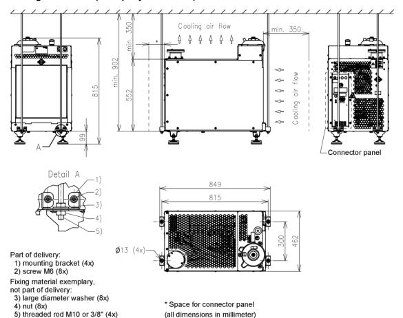
The dummy load can be installed below a solid ceiling with bearing capacity higher than 500 kg to ensure stability. The rear connector panel, emergency stop button and filling port need to be easily accessible. Do not install the dummy load close to temperature sensitive equipment. Ensure sufficient pass line heights and the required cooling air flow space, refer to floor installation.
