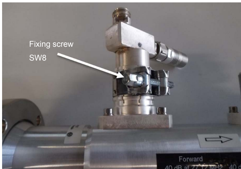
Figure 9: Fixing screw, exemplary shown for BN 800264
