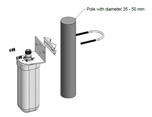
Step 3: Complete the installation by tightening the M5 nuts.
