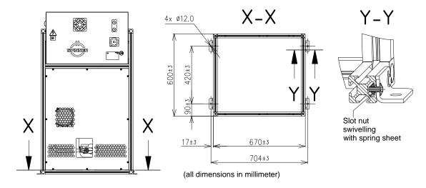
Use all 4 mounting holes of the external heat exchanger to fix it with suitable screws to the floor, or with fasteners (e.g. wall hanger supports lengths 780 mm, refer to chapter "Accessories") and screws to a wall or support structure with bearing capacity higher than 160 kg.
