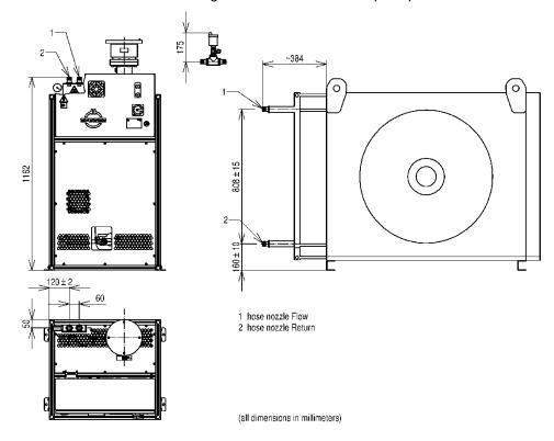
• The automatic vents must be mounted at the highest point of the cooling circuit, at least one each in flow and return. When laying hoses with several peaks, a valve must be fitted at each peak.
