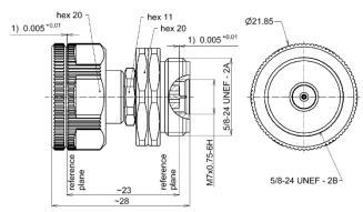
1) Pin depth (inner conductor recessed)
