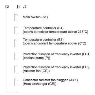
The internal interlock loop complies with the requirements for Safety Extra Low Voltage (SELV according to DIN EN 60950-1, safe separation, proof voltage resistance 3 kV AC to primary circuit).
