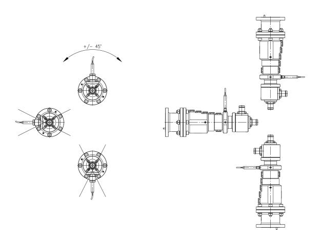
Use at least two of the mounting threads M6 to bolt the load with suitable screws to the assembly support. The quality of the screws and the tightening torque are the responsibility of the user.
