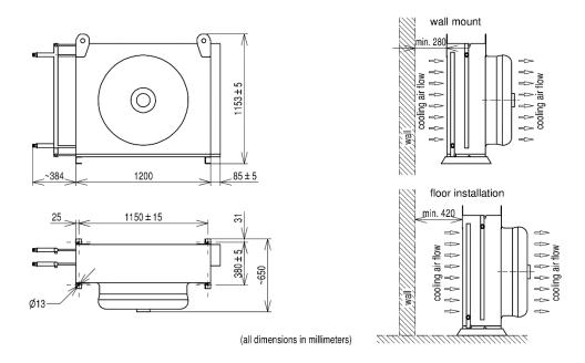
**NOTICE** Ensure unobstructed air circulation to avoid overheating. Free space on the suction side is required.
