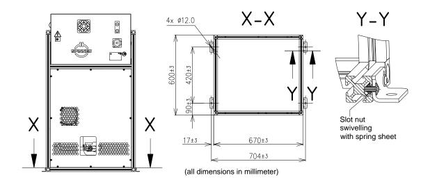
• Use all 4 mounting holes of the external heat exchanger to fix it with suitable screws to the floor, or with fasteners (e.g. wall hanger supports lengths 780 mm, refer to chapter "Accessories") and screws to a wall or support structure with bearing capacity higher than 140 kg.
