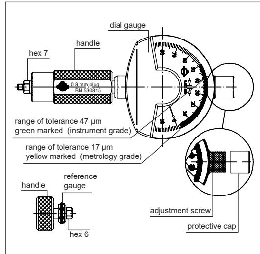
The suggested initial interval for recalibration is 12 months. The actual need for recalibration depends on the use and the maintenance of the gauge.
