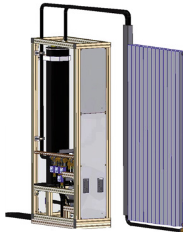
Pump unit and indoor cooler
