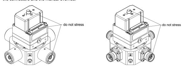
Use the fastening threads on the bottom or the lateral fastening threads to bolt the switch securely to the mounting rack. Do not clamp the RF switch on the casing. Use a torque wrench to tighten the bolted connections to 1.2 Nm (bolt material A2-50) / 2.5 Nm (bolt material A2-70).
