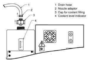
To refill, remove the cap (3), if necessary, unscrew the nozzle adapter (2) with drain hose (1) beforehand.
