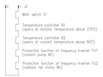
The internal interlock loop complies with the requirements for Safety Extra Low Voltage (SELV according to DIN EN 60950-1, safe separation, proof voltage resistance 3 kV AC to primary circuit).
