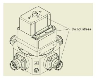
Use the lateral fastening threads or the four fastening threads on the bottom of the switch to bolt it securely to the mounting rack. Use a torque wrench to tighten the bolted connections, e.g. torque 1.7 Nm with bolt material A2-70.
