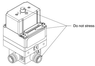
Us the lateral fastening threads to bolt the switch securely to the mounting rack. Use a torque wrench to tighten the bolted connections, e.g. torque 1.7 Nm with bolt material A2-70.
